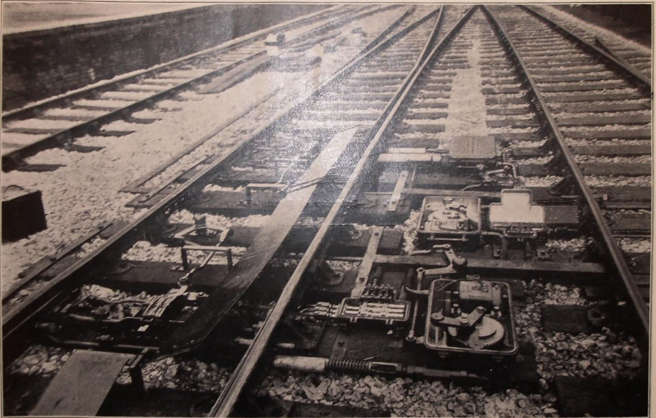
Fig. 2.—Typical Point Lay-out.
