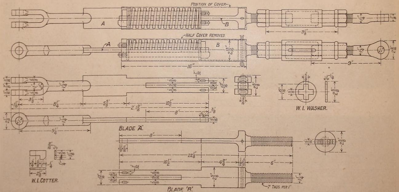
Fig. 7.—Details of Safety Spring.
