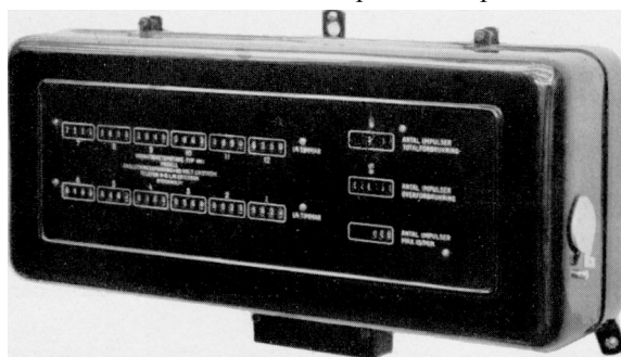
Fig. 14. Duration meter, used for summing the load of the motor-generator stations.
