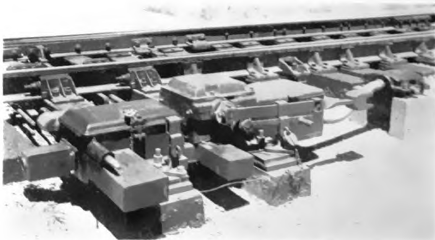
Dual-control electric switch machines at siding switches
