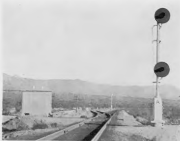
Power switch and semi-automatic signal layout at east end of Chase siding is typical
