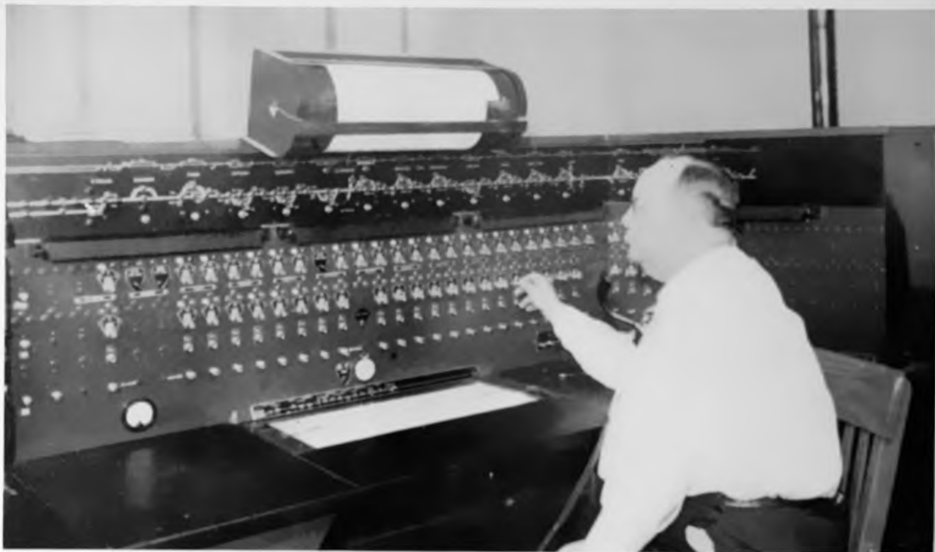
Above—The C.T.C. between East Tulsa and Afton is controlled by a machine in the dispatcher's office at Tulsa. Below—Eastbound freight train passing over the No. 20 equilateral turnout at East Tulsa
