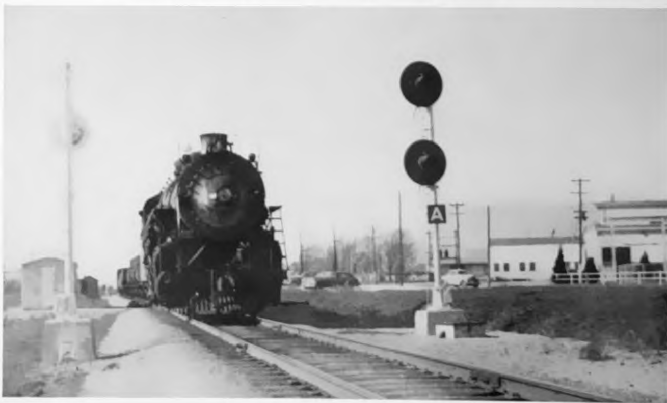
Above—The C.T.C. between East Tulsa and Afton is controlled by a machine in the dispatcher's office at Tulsa. Below—Eastbound freight train passing over the No. 20 equilateral turnout at East Tulsa
