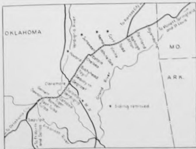
Sidings were removed at five points in the C.T.C. territory between Afton and East Tulsa
