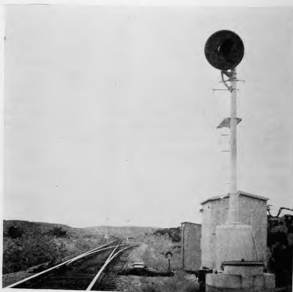
A station-entering signal and a power switch at the end of typical siding
