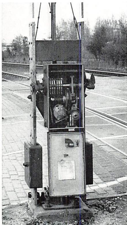
Open gear box with built-in driving mechanism of EBOH.
